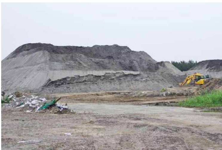
FIGURE 37 - One of three mountains of liquefaction sand in Urayasu City. Liquefaction ejecta totaled over 80,000 m 3 . (Siu)
