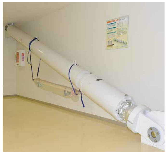
FIGURE 21 - Hydraulic Fluid Viscous damper at Tohoku University. (Swanson)
