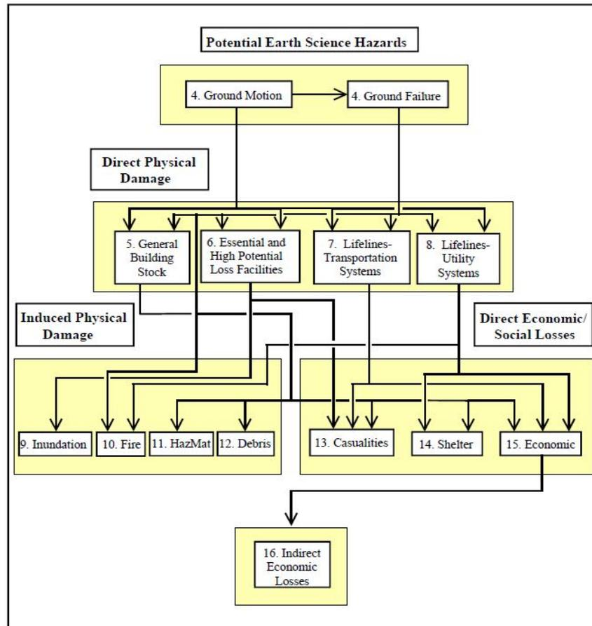
Fig. 6 – Flow Chart for HAZUS Earthquake Module [16].
